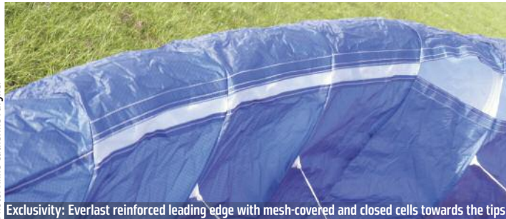
Exclusivity: Everlast reinforced leading edge with mesh-covered and closed cells towards the tips
