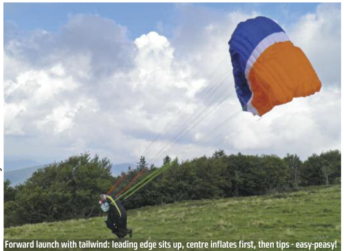
Forward launch with tailwind: leading edge sits up, centre inflates first, then tips - easy-peasy!
